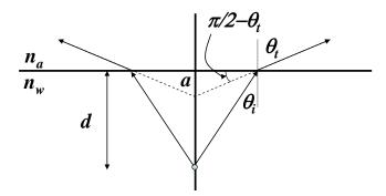
Consider the case where we are not looking directly down, but our line of sight is displaced a distance, x. Then if the real object depth is d then the apparent object depth is a. From the geometry in the picture we conclude that:
